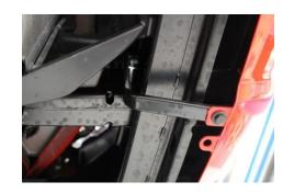
3. Insert tube spacer washer into the driver and passenger chassis holes and over the M12 bolts (from the outside).
