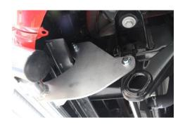
5. Driver side: Fit M8 x 130 bolt with flat washer through hole in mount plate and up through chassis. Fit M8 flat washer and M8 nyloc nut.
