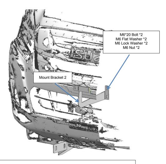
Mount Bracket 1 and Mount Bracket 2 have been installed as shown in the following figure
