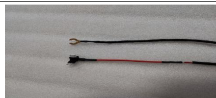
Power cable and fuse
