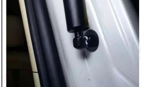
8. Install our body screw ball (same left and right)
