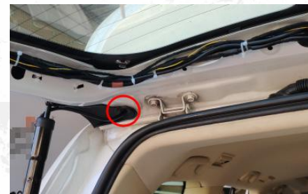
11. Insert our strut wire into the hole and plug the rubber plug (same left and right)
