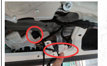
12. Unplug the original car lock wire and connect it to our wire
