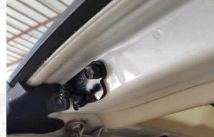
7. Use our original car screws to install our tailgate bracket(L:left,R:right)
