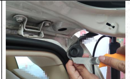
10. Cut off the waterproof rubber plug of the original (same left and right)
