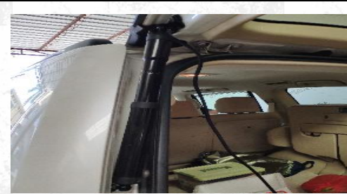
9. Install our electric pole ("L" left and "R" right)
