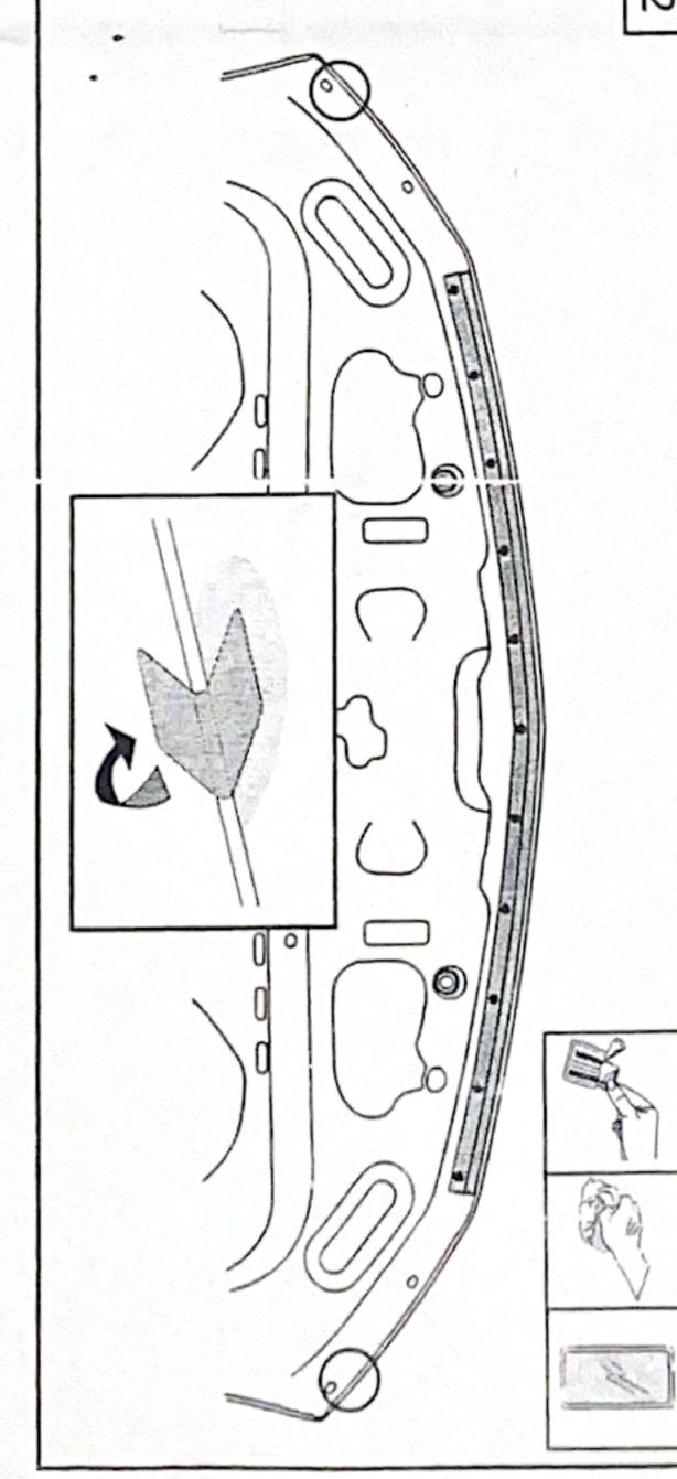
4. Slide the metal wing clips over the abrasive resistant tape strips on the hood edge at the two previously noted outer positions.
