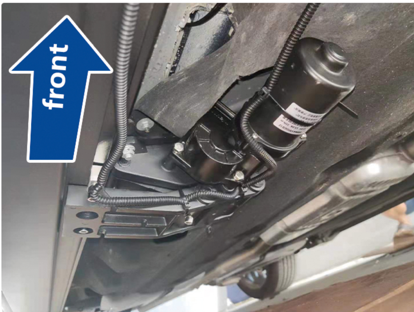
Proper method for routing light cables.
