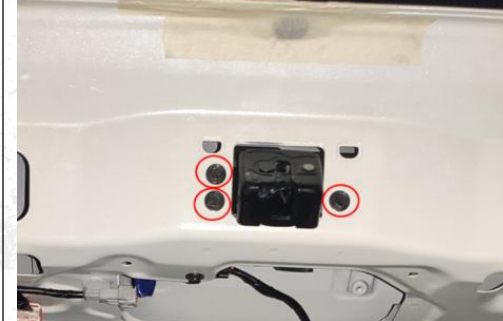
9.Remove the original lock block and replace our upper suction lock
