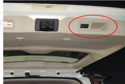
18. Use a 22mm drill bit to punch holes at the appropriate position on the tailgate and install our rear buttons
