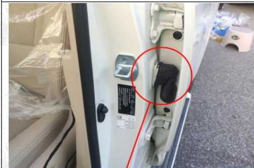
11.Locate the key at pillar B to unlock the signal cable
