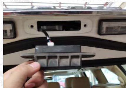
16. Unplug the original rear door button wire connect it to our wire
