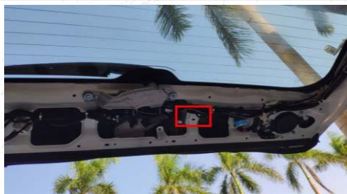
17. Connect the corresponding wiring harness to the control box and fix the control box
